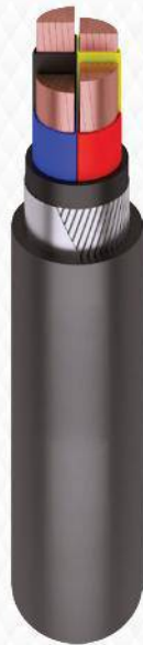
0.6/1 (1.2) kV, NYFGbY (Cu / PVC / SFA / PVC)
